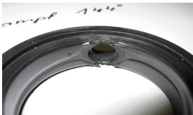
Figure 2. Swelling of the seal, with tear, in conjunction with imprecise closing of the butterfly valve.
