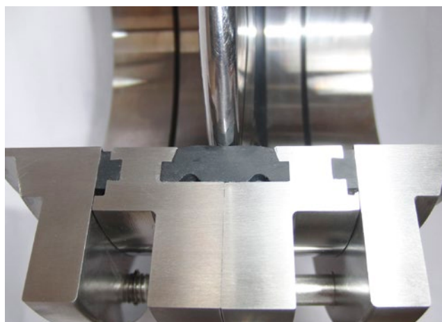
Figure 3. Cross-sectional view of a butterfly valve with optimum installation situation for the seal.
