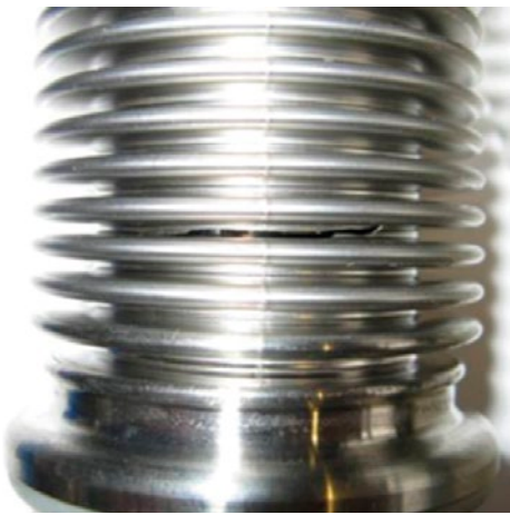
Figure 10. Damage to the bellows means that contamination is inevitable.
