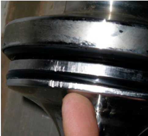
Figure 8. Traces of wear on the valve disc.
